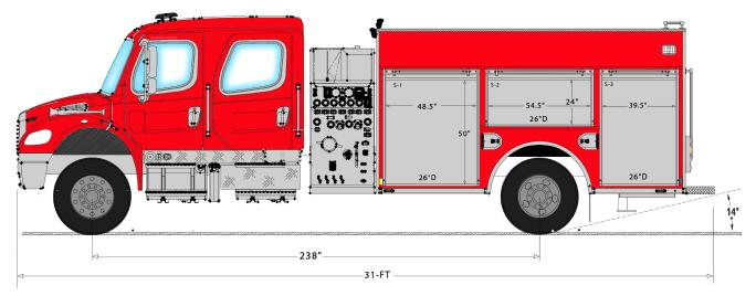
All-aluminum, huck-bolted body designed for long-term durability and maximum storage capacity. This technology provides a lightweight body without sacrificing structural integrity. The design has been verified with stringent Finite Element Analysis (FEA)where the body is stressed to the maximum chassis Gross Vehicle Weight Rating (GVWR) and off-road frame twisting to assure long-term durability.
